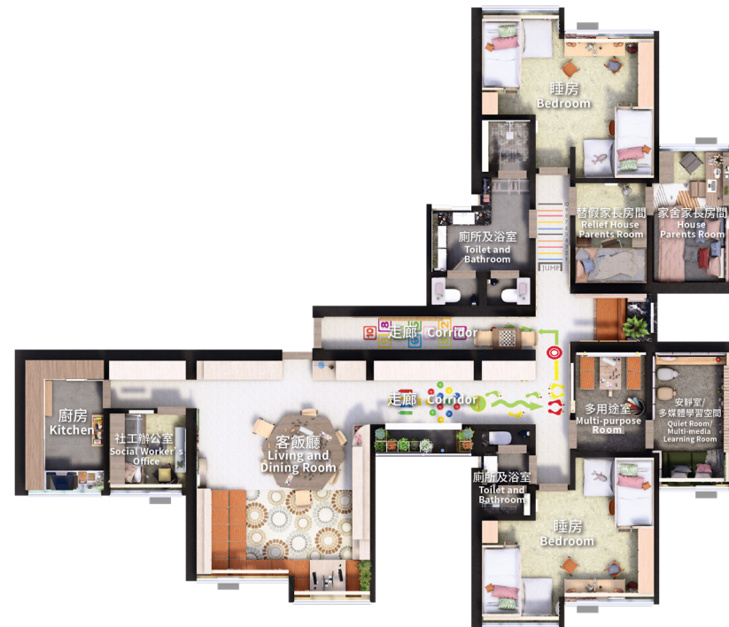
圖七：新兒童之家設計平面圖 Figure 7: Layout Plan of the New SGHs Design
